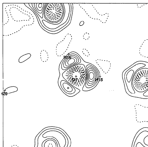
Fig. 9. Experimental deformation density in the O(7)—H(15)—H(16) plane. Contours, size and resolution as for Fig. 1.
